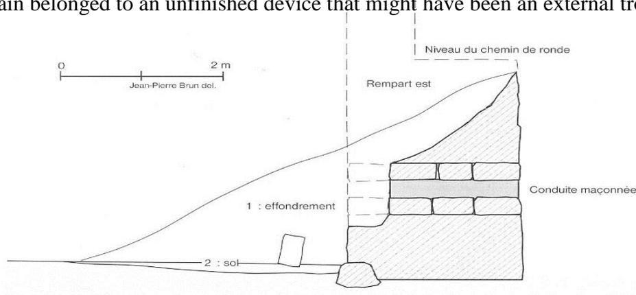
Fig. 6 A plan of the piping system through the eastern curtain After, Adam, Brun, and Redde, “Al Zarqa (Maximianon)”, Fig. 89.
