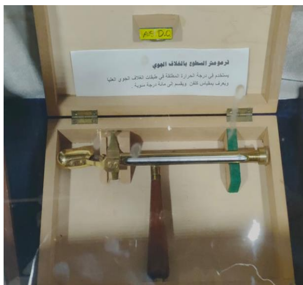
Plate. 12: The atmospheric brightness thermometer is used to measure temperatures in the upper layers of the atmosphere, photographed by the Researcher after the permission of Helwan Observatory
