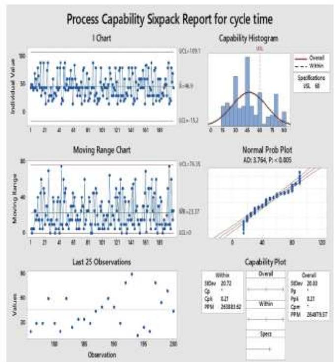
Figure 5 Process Capability Sixpack Report for cycle time
